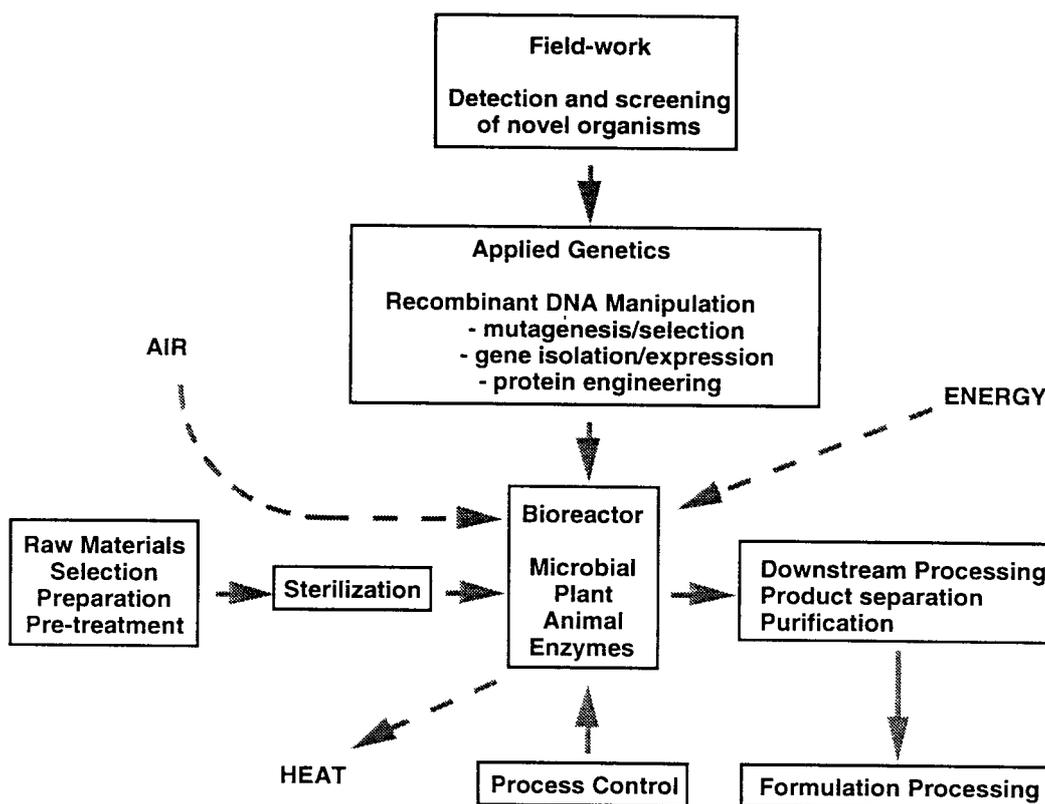
**Figure 3.** The stages of a biotechnological process. When balancing the books, it must not be forgotten that a crucial part of the input is research and development. Often R & D can take many years before a process becomes feasible or cost effective.
