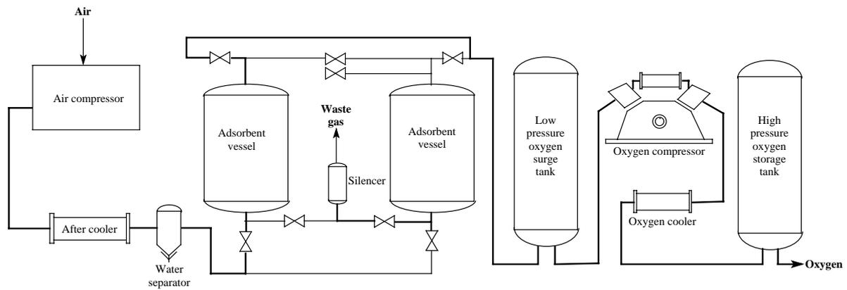
**Figure 2 - Schematic representation of the PSA process**
