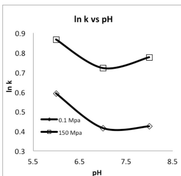
**Fig. 4.** The pH profile for the hydrolysis of cytosine at 0.1 MPa and 150 MPa. pH values shown at 150 MPa are those corrected for pressure effects. It can be seen that there is a minimum in the rate of hydrolysis just above pH 7. The lines are for visual reference only.
