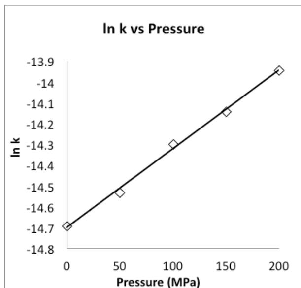
**Fig. 3.** Plot of the log of the rate constant  $k$  for the hydrolysis of cytosine vs. pressure  $p$ . From the slope of the line  $-\Delta V^\ddagger/RT$  the activation volume  $\Delta V^\ddagger$  can be derived.
