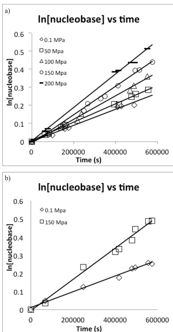
**Fig. 2.** Plot of  $\ln$  [nucleobase] vs time at 373 K for (a) cytosine at various pressures and (b) cytidine at 0.10 MPa and 150 MPa. The rate constant for hydrolysis of cytosine to uracil is given by the slope of the fitted line
