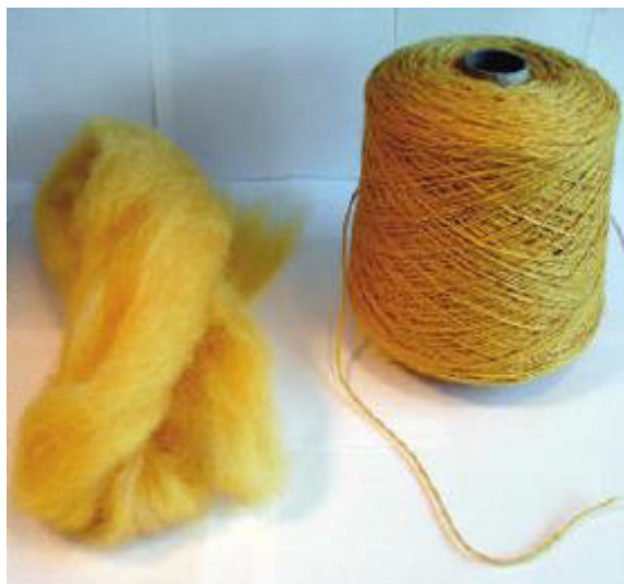
Fig. 5. Nanosilver–wool fibre composites produced with yellow AgNPs. Reproduced with permission from ref. 17. © 2011 American Chemical Society.
