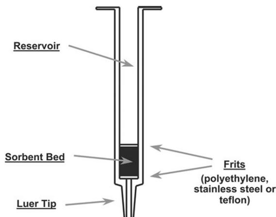
Fig. 1. Typical SPE column [adapted from ref. 7]
