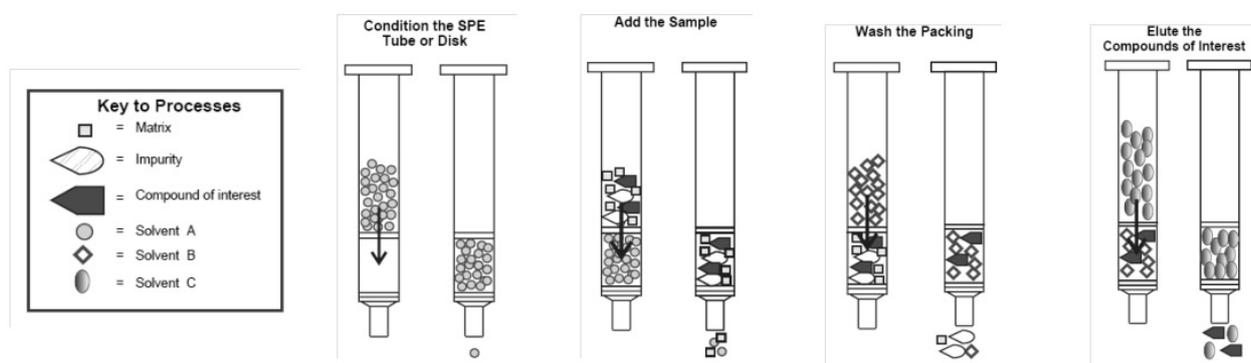
Fig. 2. The solid phase extraction process [adapted from ref. 5]
