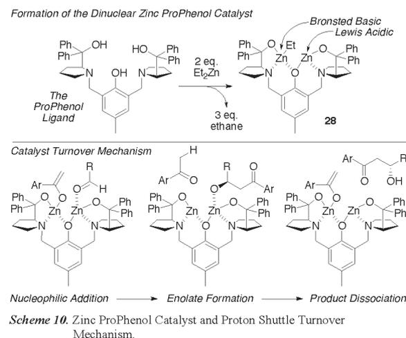
Scheme 10. Zinc ProPhenol Catalyst and Proton Shuttle Turnover Mechanism.
