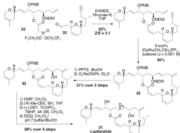
PPTS = pyridinium *p*-toluenesulfonate, DET = diethyl tartrate, TBHP = *tert*-butyl hydroperoxide, DDQ = 2,3-dichloro-5,6-dicyano-1,4-benzoquinone.
