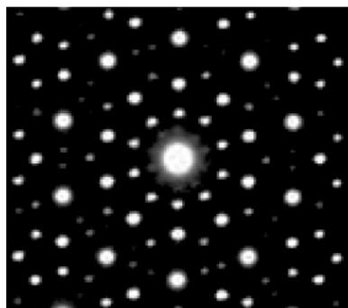
**Fig. 1.** Shechtman's ten-fold diffraction pattern; rotating the image through  $36^\circ$  results in the same pattern (adapted from *Scientific Background on the Nobel Prize in Chemistry 2011*, with permission from The Royal Swedish Academy of Sciences; [www.nobelprize.org/nobel\\_prizes/chemistry/laureates/2011/info.htm](http://www.nobelprize.org/nobel_prizes/chemistry/laureates/2011/info.htm)).
