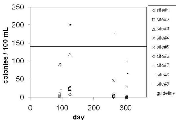
Fig. 9. *Enterococci* count variation at each site during 2009; samples with colonies too numerous to measure are shown as 200 colonies/100 mL.
