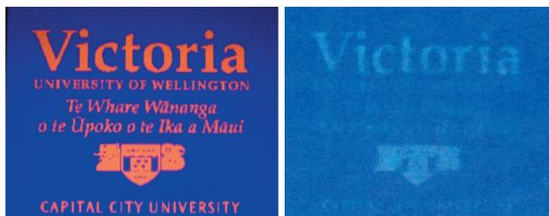
**Fig. 4.** Ink-jet paper printed logo with two passes of  $Mn^{2+}$  doped quantum dots (left) and with one pass of  $Cu^{2+}$  doped quantum dots (right) viewed under UV light – see ref. 3.
