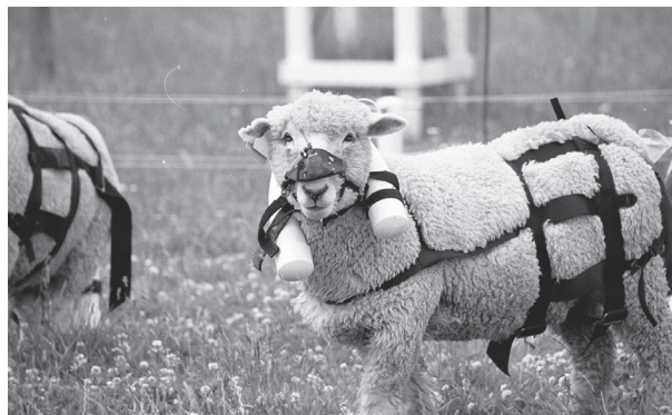
Fig. 1. Measuring gas emissions from sheep
