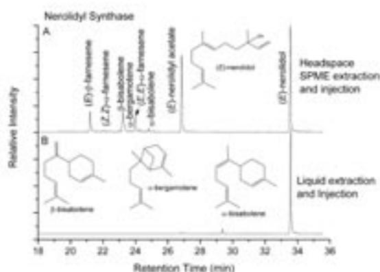
**Fig. 2.** GCMS following A) thermal desorption from an SPME fibre, and B) hot splitless injection of a solution of nerolidol into the GC injection port
