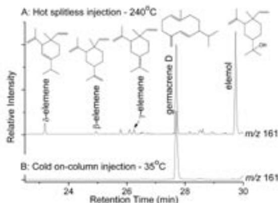
Fig. 1. Thermally labile analytes analysed by A) hot splitless GC injection, and B) cold on-column injection of a solution of germacrene D into the GC injection port
