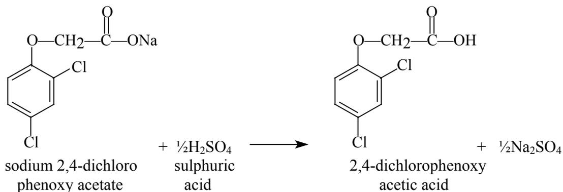
The small amount of undesirable components that remain in the xylene layer after the acidification are removed with two water washes.
