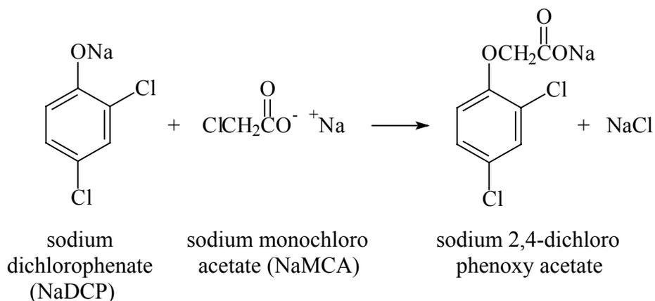
Unwanted side reactions do occur but are kept to a minimum through the choice of optimum operating conditions. NaMCA and water undergo a reaction that produces sodium glycollate and hydrochloric acid.
