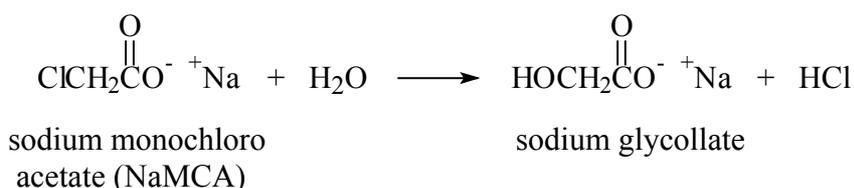
Due to the alkaline nature of the reaction mixture, any HCl formed is immediately neutralised with caustic soda to sodium chloride and water. NaMCA also reacts with caustic soda to produce sodium glycollate and water. For this reason the stoichiometric ratio of MCAA and caustic soda is strictly controlled to avoid build-up of excess caustic soda.
