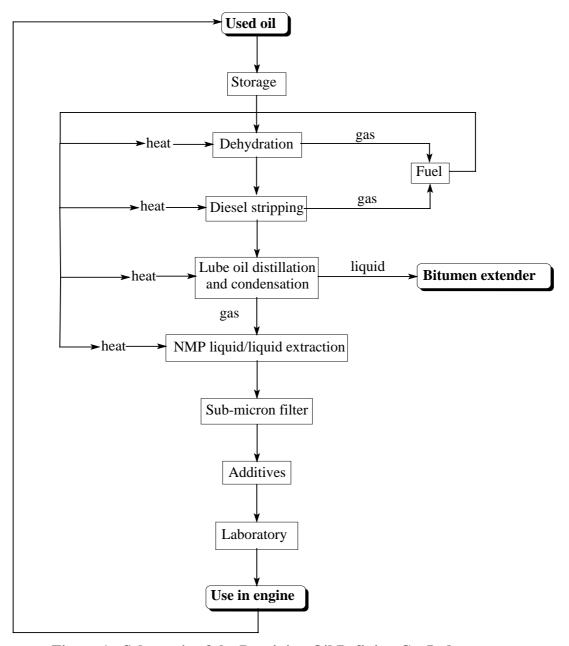
Figure 1 - Schematic of the Dominion Oil Refining Co. Ltd. process
