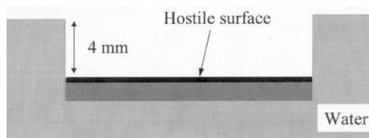
Fig. 5. Metal foil with a superhydrophobic top surface displacing more water than its volume.
