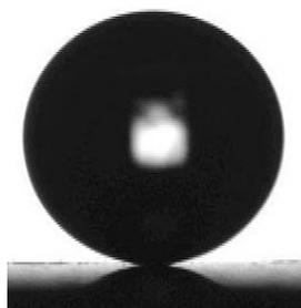
**Fig. 3.** An  $8 \text{ mm}^3$  water droplet on zinc coated with silver, coated with polyfluoroalkylthiol.
