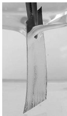
**Fig. 4.** Underwater mirror revealing blemishes (upwards from bottom left).
