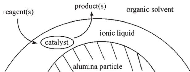
Fig. 5. Schematic of supported ionic liquid phase catalysis (SILPC).
