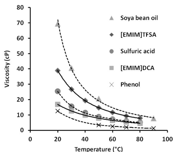
**Fig. 3.** Plot of viscosity versus temperature for  $[\text{EMIM}]\text{TFSA}$ ,  $[\text{EMIM}]\text{DCA}$  and some common liquids.
