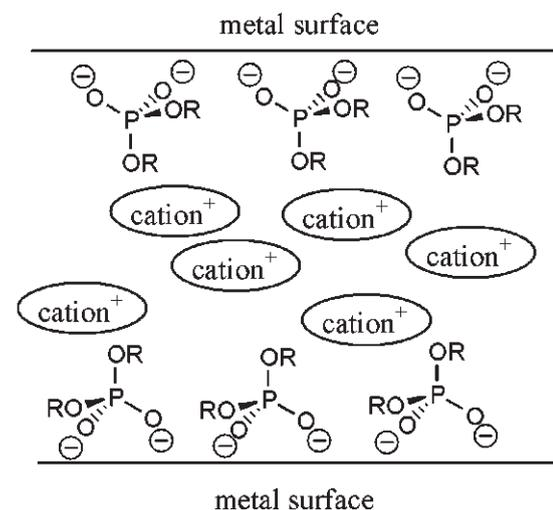
Fig. 4. A phosphate IL between two metal surfaces.
