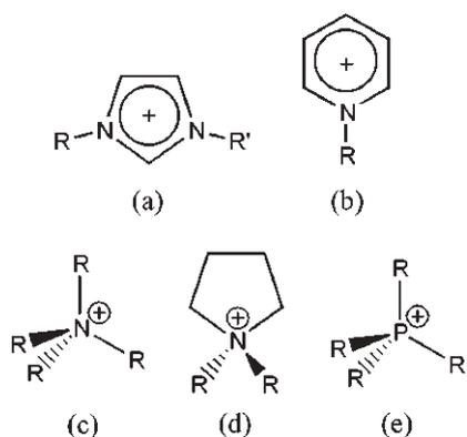
**Fig. 1.** Common classes of cations used in ILs: (a) imidazolium, (b) pyridinium, (c) ammonium, (d) pyrrolidinium and (e) phosphonium.
