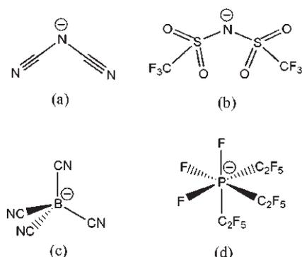
**Fig. 2.** Common anions used for ILs: (a) dicyanamide (DCA), (b) bis(trifluoromethanesulfonyl)amide (TFSA, TFSI or  $\text{NTf}_2^-$ ), (c) tetracyanoborate and (d) tris(pentafluoroethyl)trifluorophosphate (FAP).
